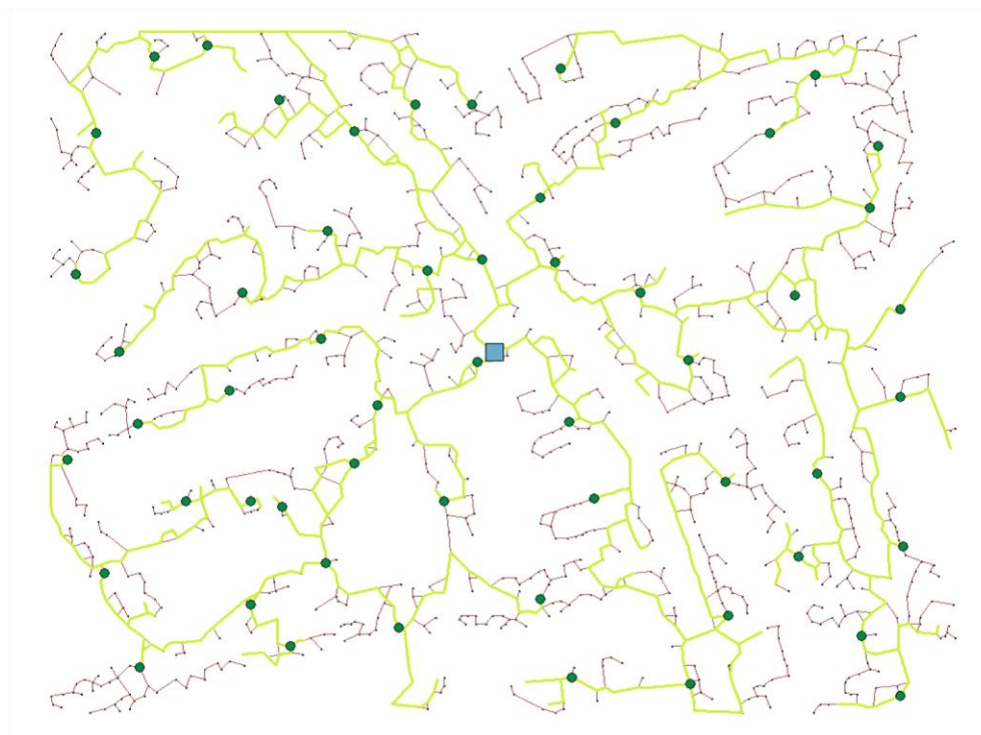
Figure 26, exemplary urban network for Germany. The blue square marks represent the location of the HV/MV substations, the green lines represent the MV network delineation, the green dots represent the location of MV/LV transformers and the purple lines represent the LV network.
