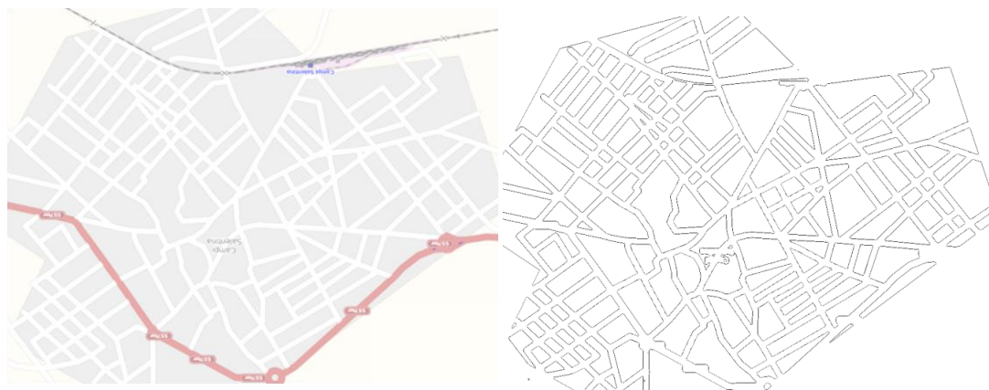
Figure 44, example illustration of the identification of the street contours in an image of certain location taken from Open Street Map to locate network users and geographical constraints
