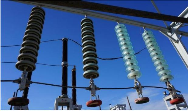
**Fig. 3.** Test set-up. From left to right: full-coated, half-coated, non-coated and nano-coated glass insulators.
