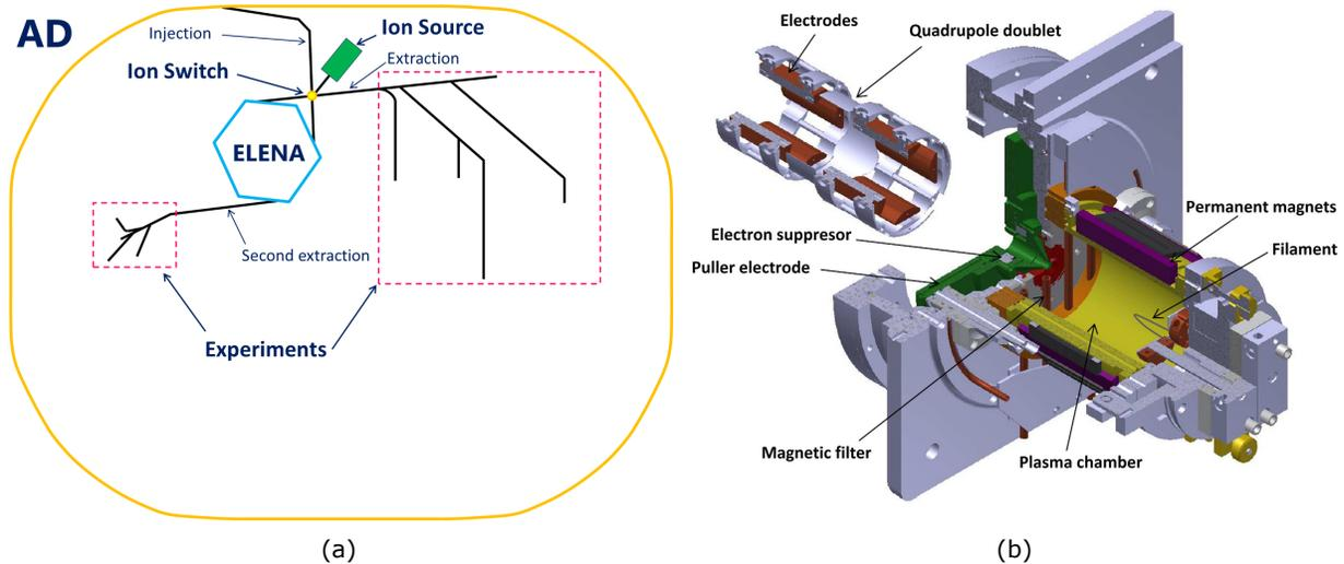
**FIGURE 1.** (a) AD Hall Layout. The yellow outer lines marks the AD path. Inside it the ion source, ELENA ring and the main experimental lines are shown. (b) Ion Source section view
