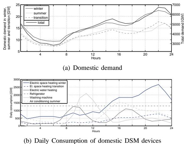
Fig. 1. Electricity consumption of households in (a) and domestic DSM devices in (b)
