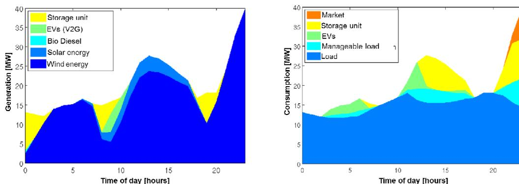
**Figure 2.3 - Power injection into the VPP and power extraction from the VPP for August 15 in Scenario 2009**
