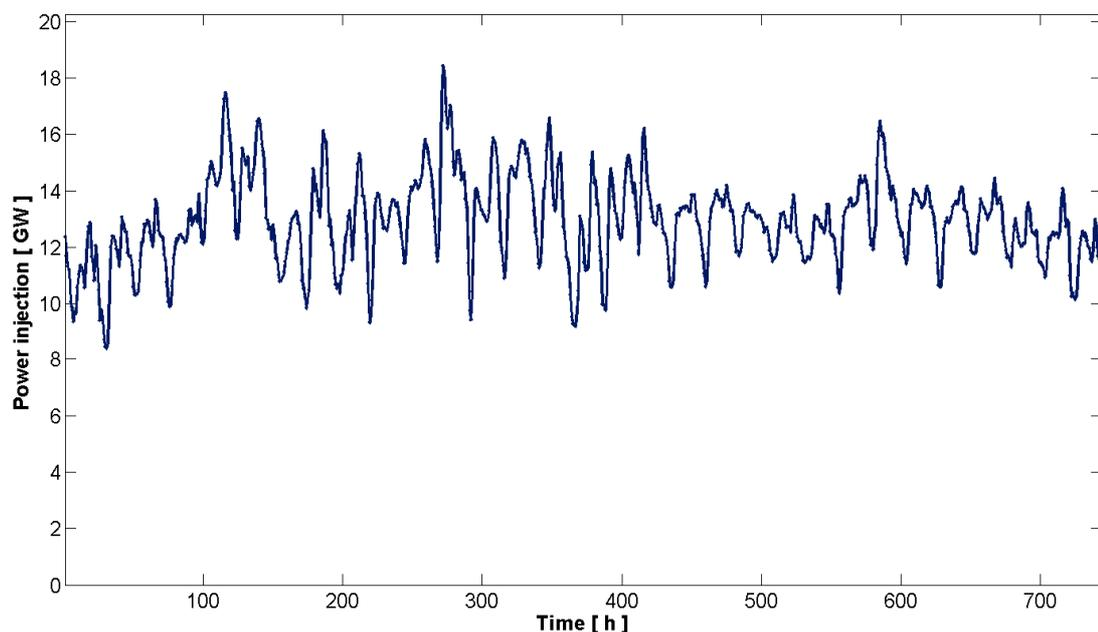
**Figure 2.1 - Power injection in East Germany - 50Hertz Transmission area: period under consideration: 01.01.2011 - 31.01.2011**
