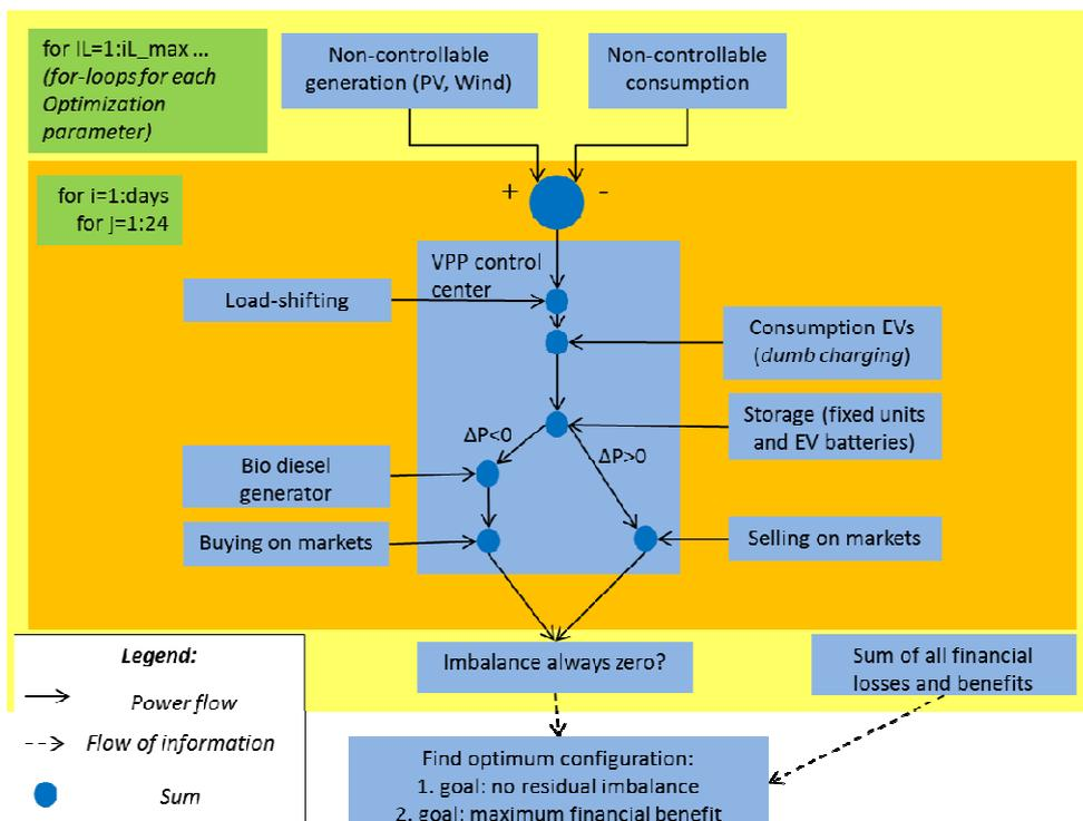
**Figure 2.2 - Basic structure of balancing algorithm**
