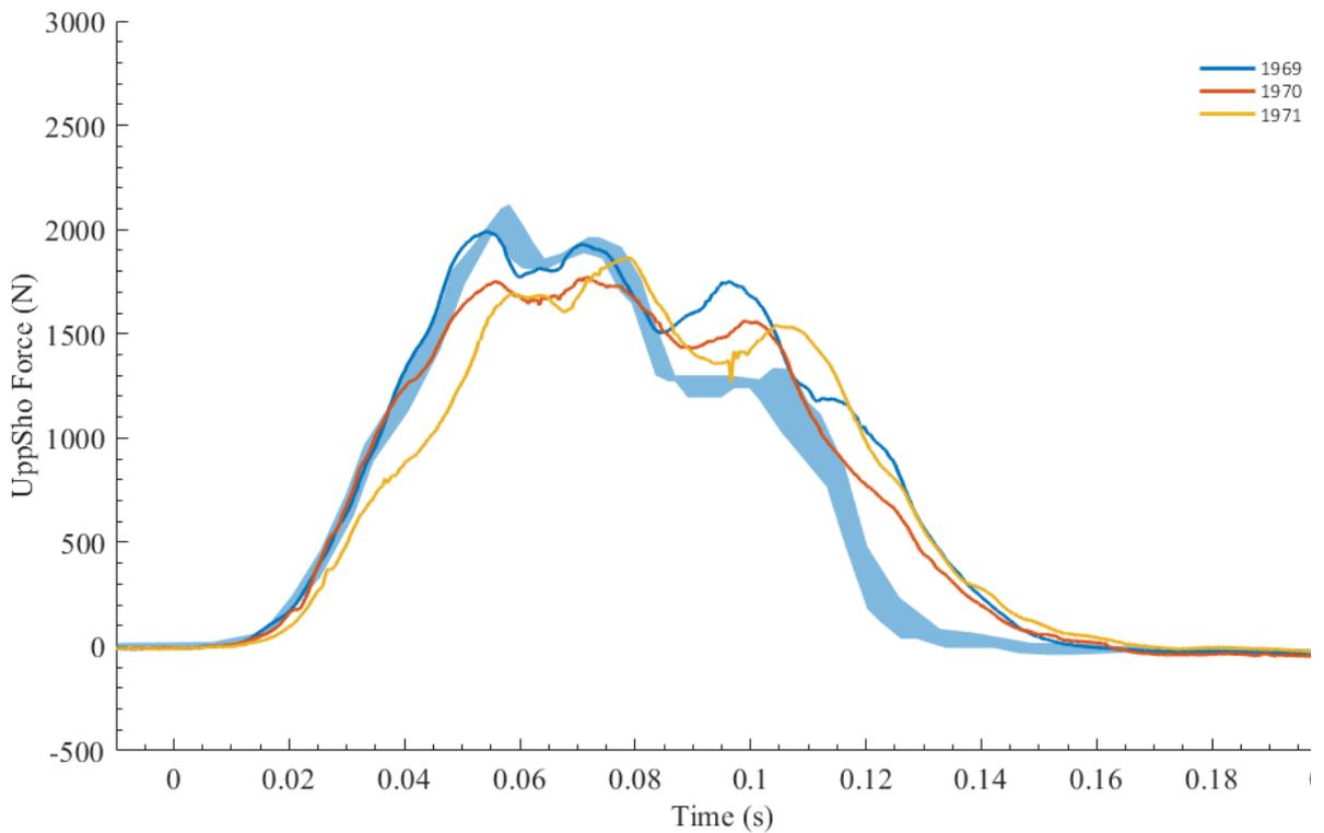
Figure 1 Time history of the upper shoulder seat belt force. Top: first series of PMHS tests (solid lines) and corridor response of corresponding THOR tests (shaded blue area). Bottom: second series of PMHS tests (solid lines) and corridor response of corresponding THOR tests (shaded blue area).
