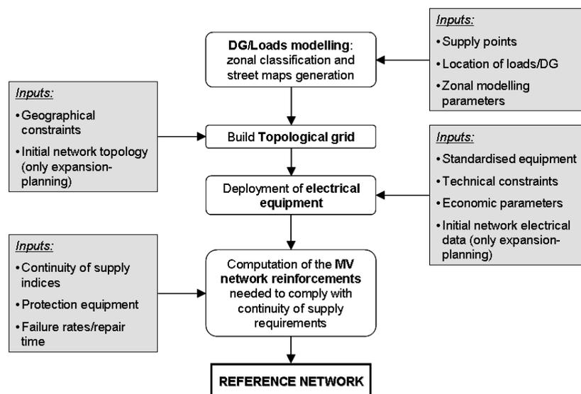
**Figure 6: Logical architecture of RNMs: steps involved and relevant input data**
