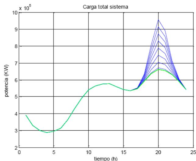
**Figure 9: Load profile (kW vs hour of the day): battery charging at home during evening hours**
