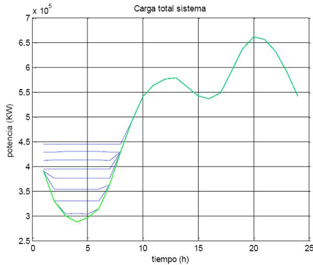
**Figure 10: Load profile (kW vs hour of the day): battery charging at home during night hours**
