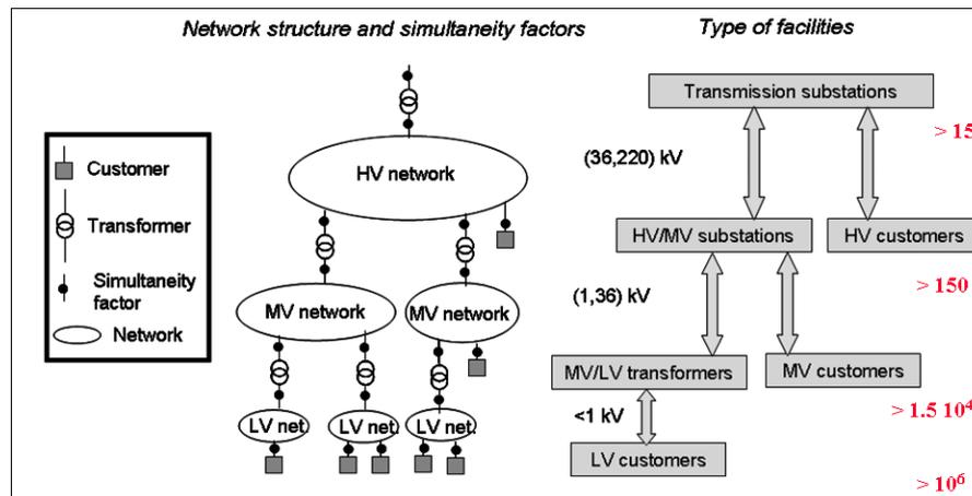
**Figure 1: Distribution network structure and simultaneity factors**
