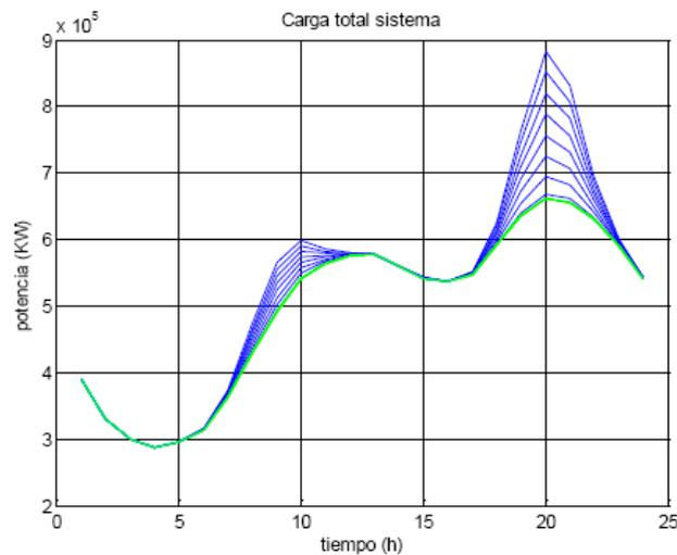
**Figure 11: Load profile (kW vs hour of the day): battery charging at home during evening hours and at work in the morning**
