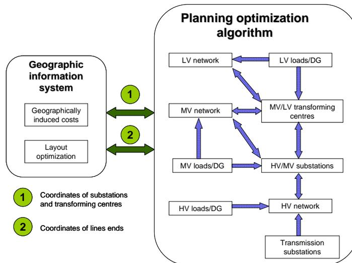
**Figure 2: Interaction between the planning algorithms and the GIS**
