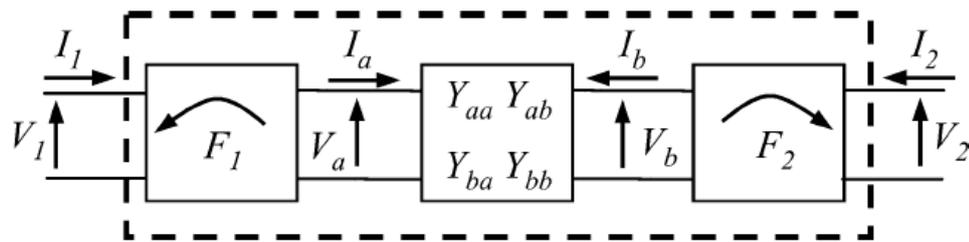
Figure 7: Two-port power flow model including simultaneity factors F1 and F2
